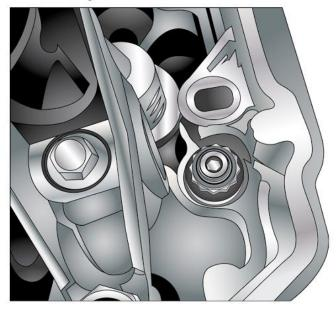
Finished machining should allow easy removal and installation of the head stud.
